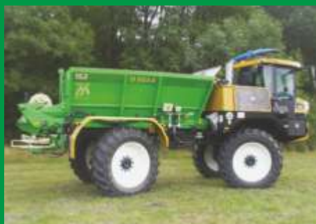
Mounted spreader on Rogator.
