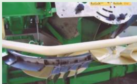
Border spreading with deflector II, switched - on.
