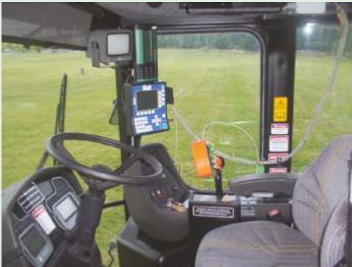
Computer over serial interface connected with external - electronics (Precision Farming).
