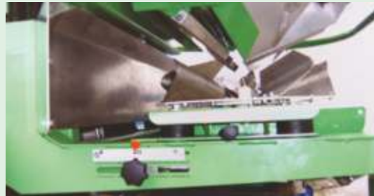
Spreading table „fore & aft“ adjustment without tools.
