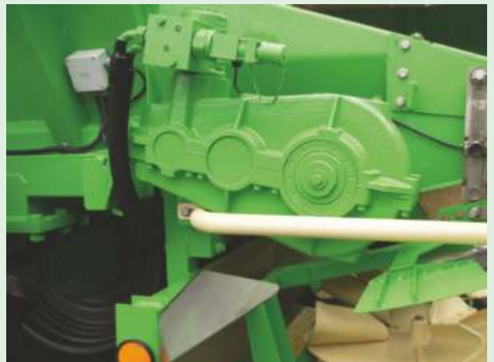
Hydraulic power is transmitted to the scraper chain system by a heavy duty gearbox. An electronic proportional valve adjusts the speed as required.
