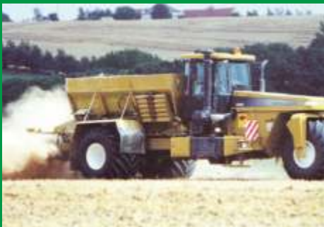
Mounted spreader on Terra Gator.
