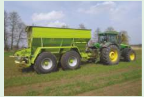
GDK 8.000 T (14 m³) with bogie axle for lime - and fertilizer spreading.
